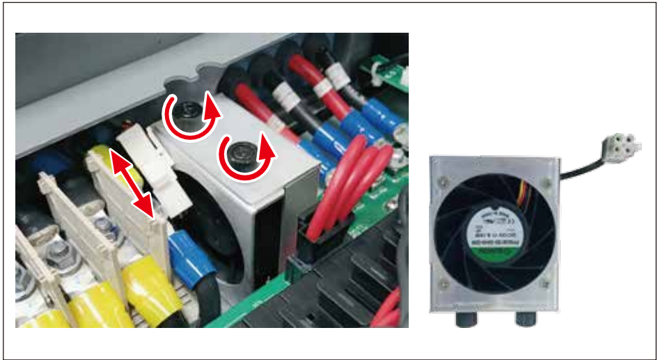
图5-8：拆卸配线箱区块之智慧风扇 (仅M88H_122)
