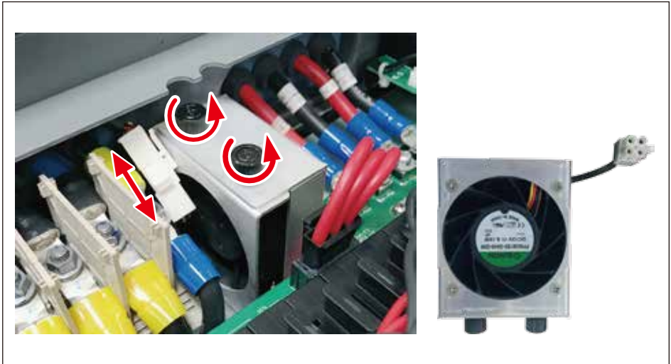
Figure 5-8 : Disassembling fan inside the wiring box compartment (M88H_122 only)
