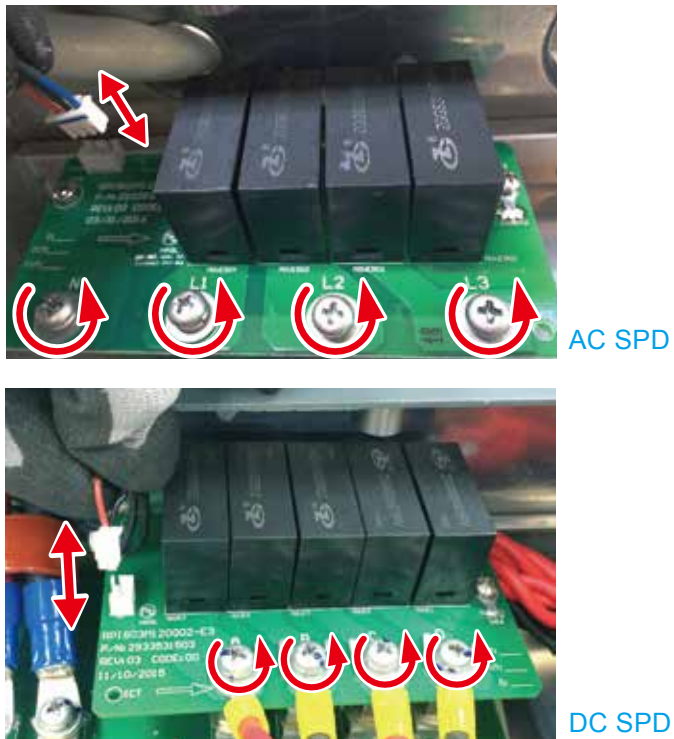
Figure 5-4 : Pull out the connectors and remove the screws as shown in arrows
