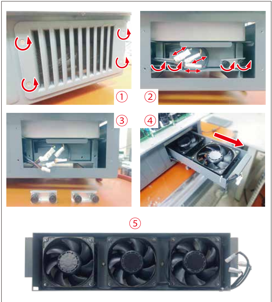
Figure 5-9 : Disassembling fans inside the power module compartment (showing one side only)
